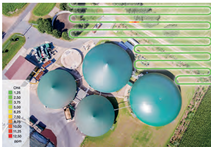
Figure 5: Even very low CH4 concentrations can be detected by scanning a biogas plant area with a drone
