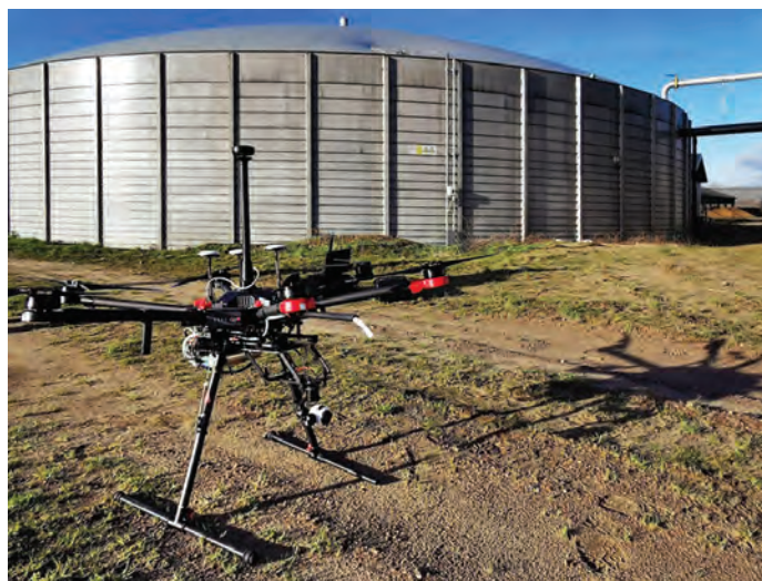
Figure 4: The LGD Compact integrated in a drone for portable UAV Leak Detection by the Danish Company Explicit
